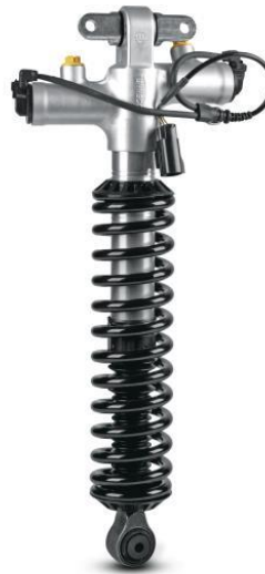
Fig. 8 Semi active suspension Volvo XC90. [14]
