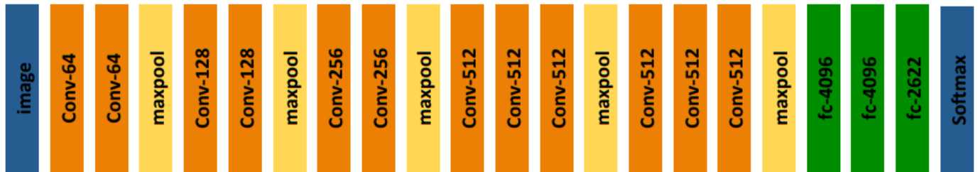
Figure 2.13: VGGFace architecture, taken from [88]. This network expands the representation every two convolutional layers, after the max pooling operation, then flattens the representation to a 4096-D face descriptor.
