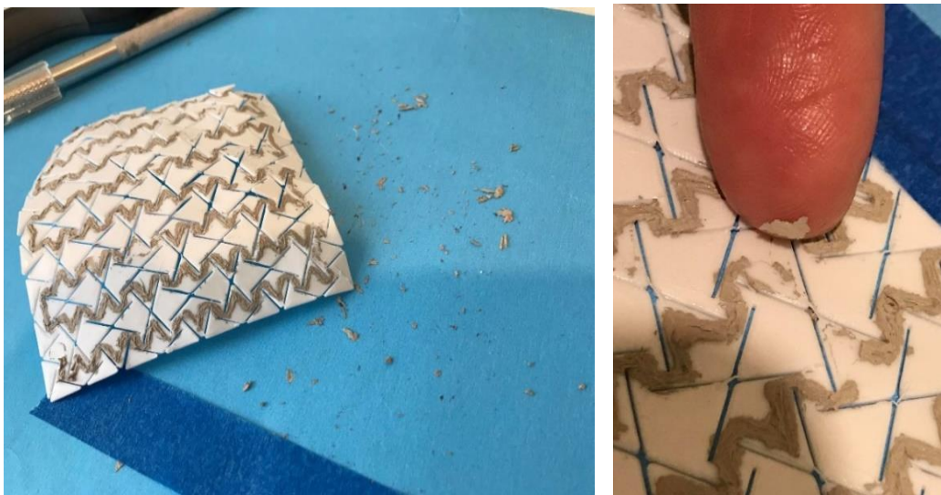
Fig. 3-17 Conductive ink was detached after bending the printed object
