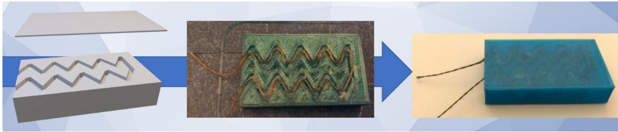
Fig. 3-32 Printing process paused to embed the conductive thread.
