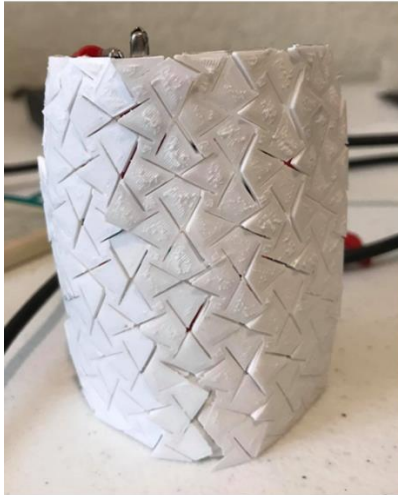
Fig. 3-23 When partial folding took place, the phase was nearly -74 degrees at 10kHz.
