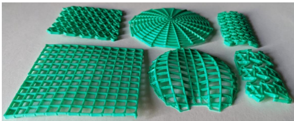
Fig. 3-13 Different trajectories generated on analytical surfaces using a conventional Ender-3 printer.
