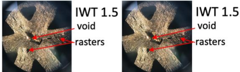
Figure 12. Details of defects in the reticle of the specimens.
