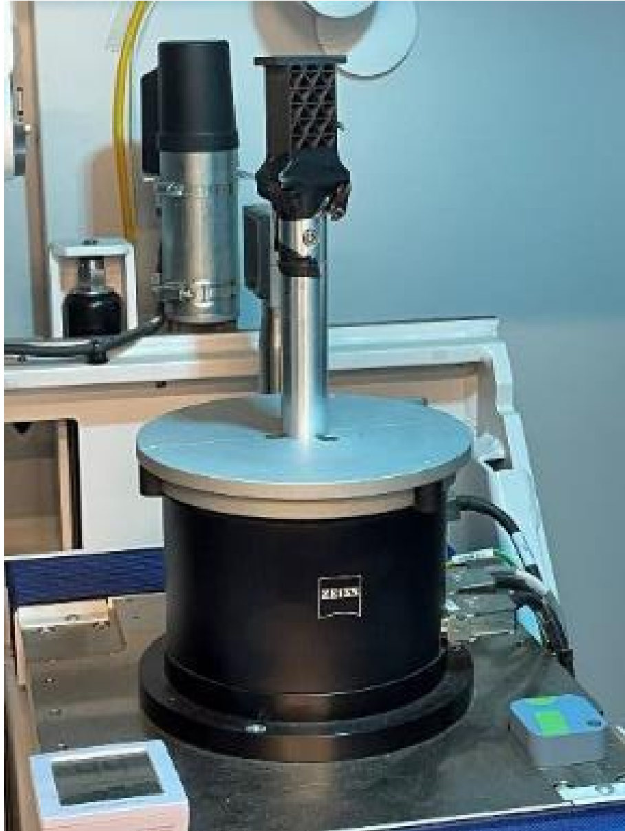
Figure 14. Specimen mounted on Metrotom 800 CT-Scan
