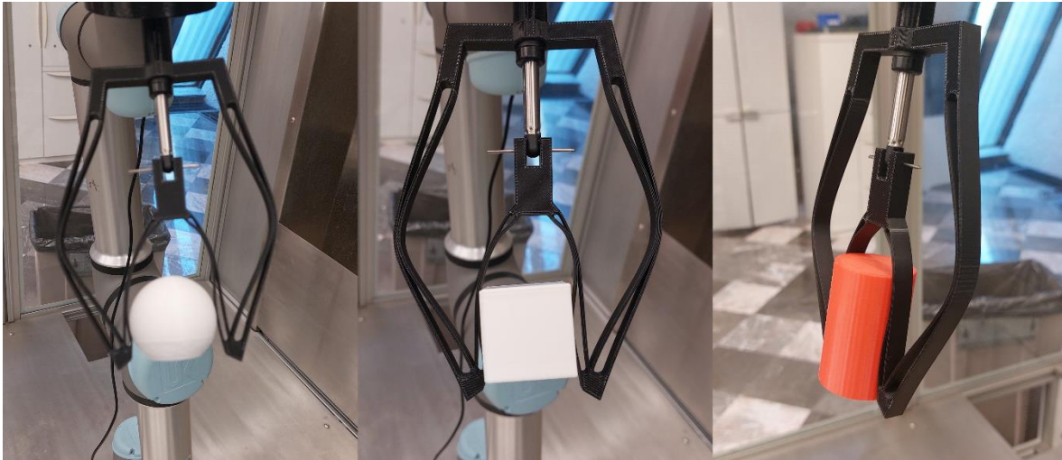
Figure 24 Gripper Model G2 - 140/17.5 - T10 – 140 mm grasping a partial sphere, a cube, and a cylinder.
