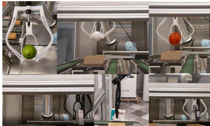
Figure 25 Grippers successfully grasping objects. From right top to left bottom: Lemon, egg, tomato, Fluoxetine, QUAL®, and Fluoxetine medicine boxes.
