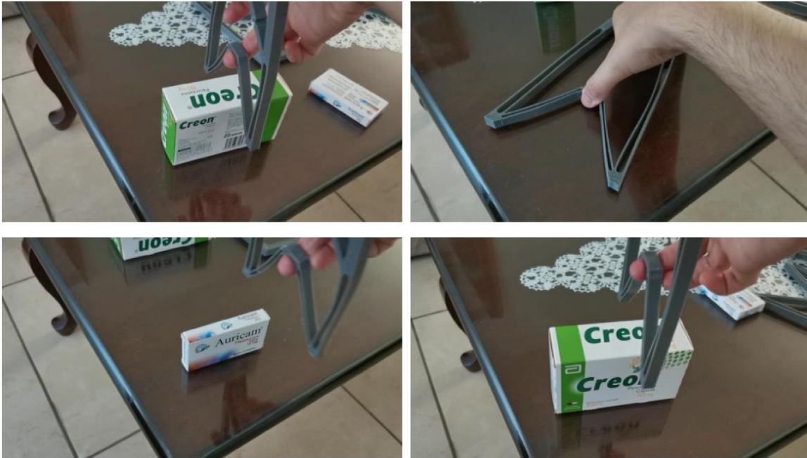
Figure 11 Manual testing of the grippers with medicine boxes
