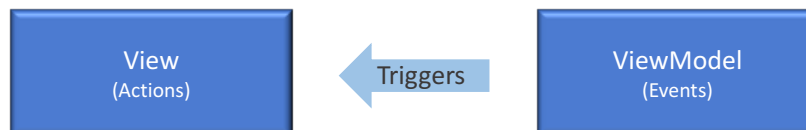
Fig. 12 View handling notifications from the ViewModel.
