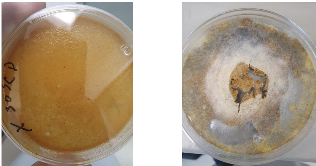
Fig. 13. SSF of tomato pomace using R. oryzae BIOTEC00X after 1 day of incubation (left) and after 7 days of incubation (right).
