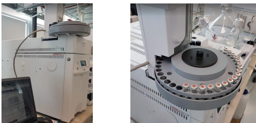
Figure 8. Gas Chromatograph used in SCFA analysis (Agilent Technologies 6850).
