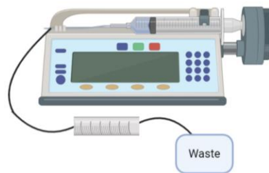
Figure 2C. Combination number 2. It integrates the syringe pump, DAQ internal control system and glass syringe as incubation chamber
