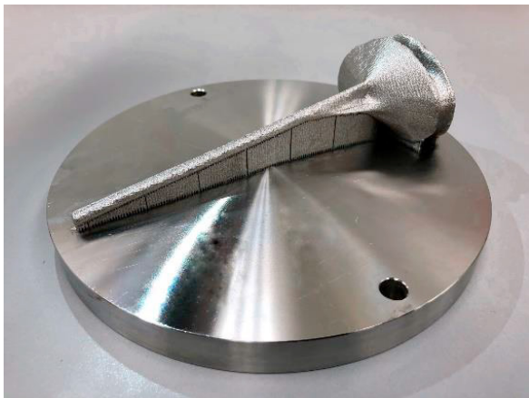
Fig. 9 Stainless steel 316L optimized tibia intramedullary implant fabricated via selective laser melting process.
