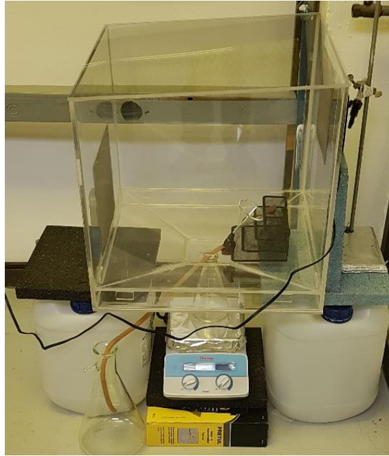
Fig. 49. The condensation chamber created and mounted for experiments analyzing the dew-enhancing efficiency of created hybrid surface pieces.
