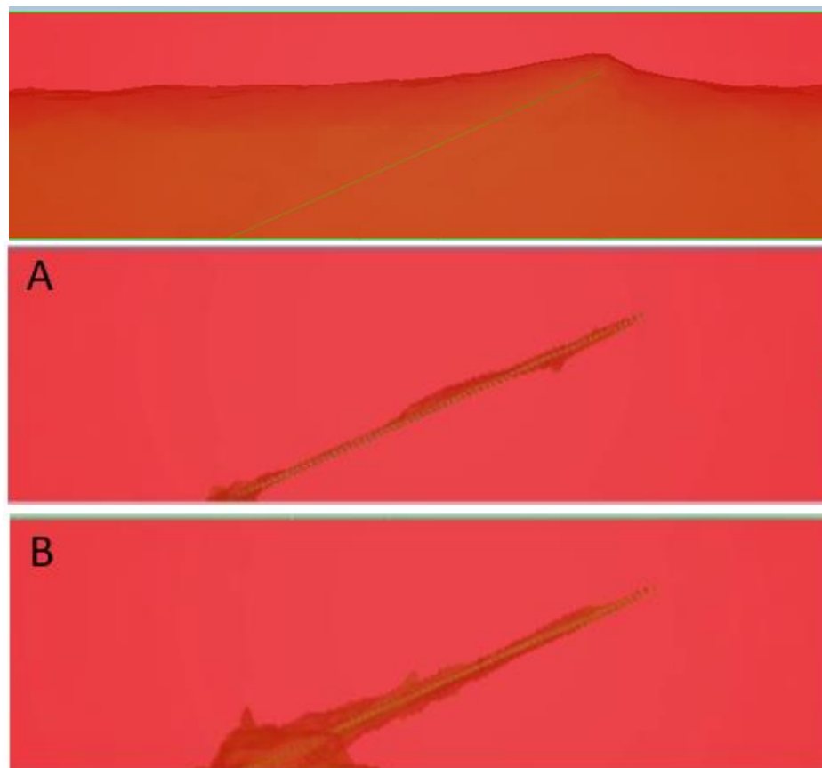
Fig. 56. (Top) Initial conditions for both simulations. (A) Computer Fluid Dynamics (CFD) simulated by the occurrence of condensation in the medium by the scalar parameter with a concave topology of the hexagonal geometry. (B) Computer Fluid Dynamics (CFD) simulated by the occurrence of condensation in the medium by the scalar parameter with a protruding topology of the hexagonal geometry.
