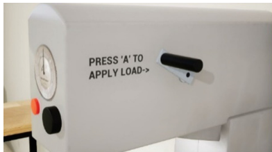
Fig. 3. Step-by-step sequence example: instruction to apply the main load.
