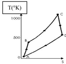
Fig. 1 Temperature as a function of Entropy in the Closed Brayton Cycle
