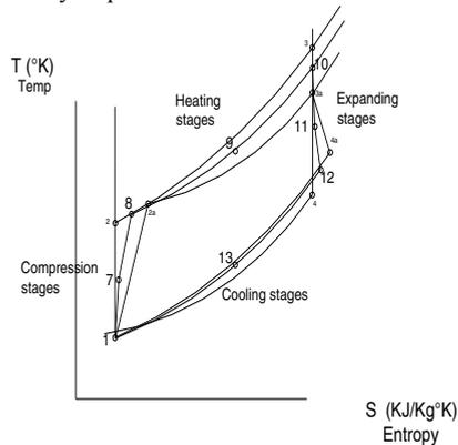
Fig. 5 Multiple stages Real Closed Brayton Cycle  $T=f(S)$
