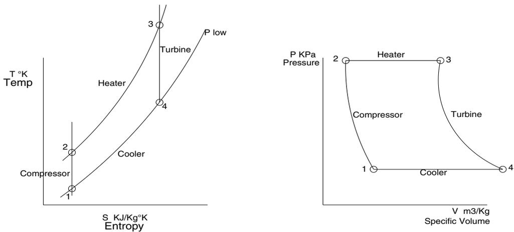
Fig. 3 Ideal Closed Brayton Cycle ( $T=f(S)$  and  $P=f(v)$ )
