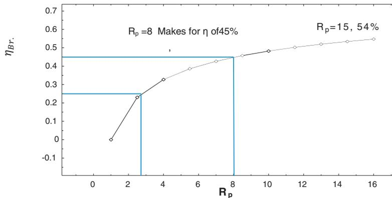
Fig.6 Brayton Cycle Overall Efficiency as function of Pressure Ratios
