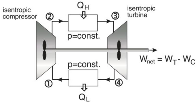
Fig. 2 Ideal Brayton Closed Thermal Engine configuration
