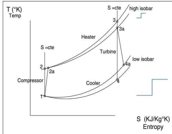
Fig. 4 Real Closed Brayton Cycle  $T=f(S)$
