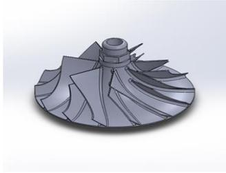
Fig 8 Modeled compressor rotor.
