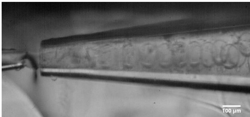
Figure 4.15 Optical micrograph showing a typical production of monodisperse double emulsion drops containing dendrimers in the oil phase.
