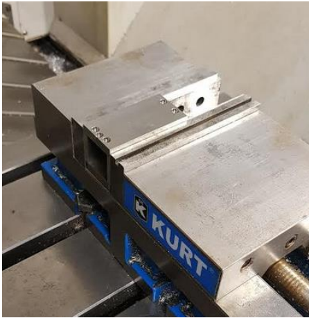
Figure 15. Kurt Clamp with Titanium block
