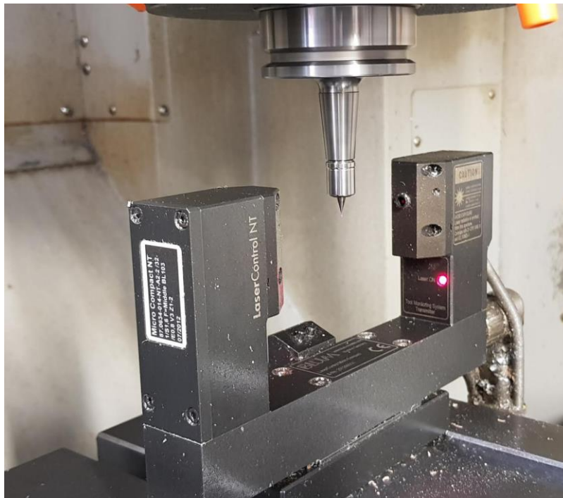
Figure 18. Blum Laser for measuring tools height
