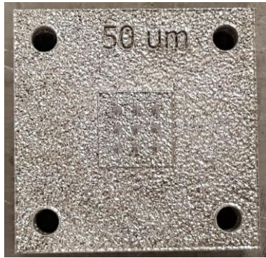
Figure 49. SLM array in Stainless Steel 316L
