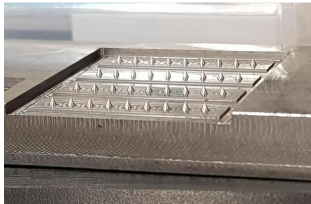
Figure 30. 4 probes machined with high and medium feed
