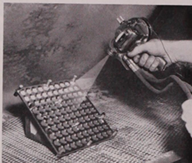
Fig. 6 — Metallizing gun in operation for applying electrodes of copper or tin to varistors.
