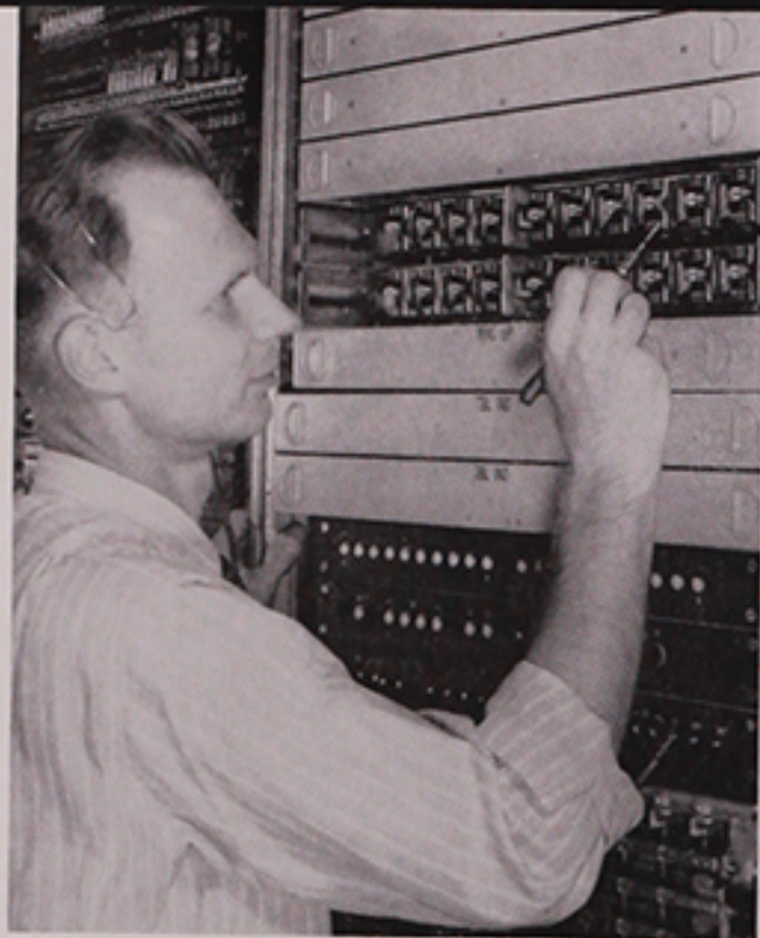
Fig. 2—F. R. Lehman of the New York company tests relay operation in concentrator equipment.
