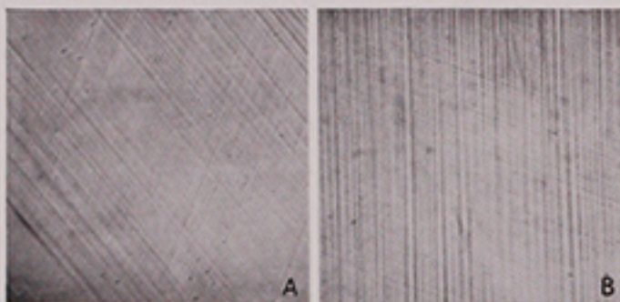
Fig. 2—Slip lines on an exposed surface of (A) crystal compressed at 525°C and (B) crystal twisted at 600°C. Magnification 75 diameters.
