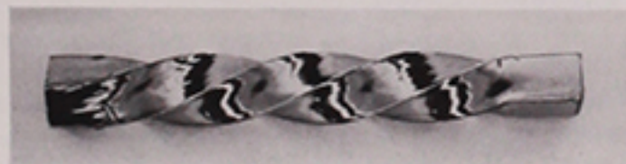
Fig. 1—Crystal of germanium twisted at 850°C.
