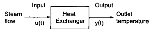
Figure 2.6: Single-input single-output continuous dynamic system. The outlet temperature is the output variable, and the steam flow is the input variable
